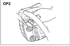
2. Continuously push the priming bulb until fuel comes in the bulb. (OP2)
